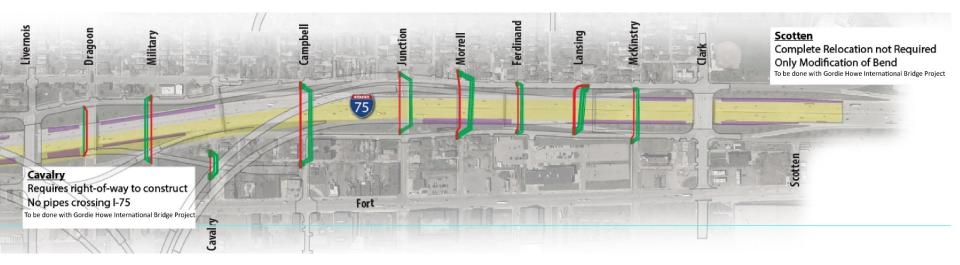
The locations of siphons and combined sewer crossings which will have their pipes under I-75 mainline pavement installed as part of the Inlay Project.
