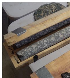
Core samples taken from the Canadian bridge tower site
