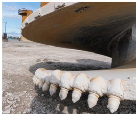
Drill teeth attached to an auger
