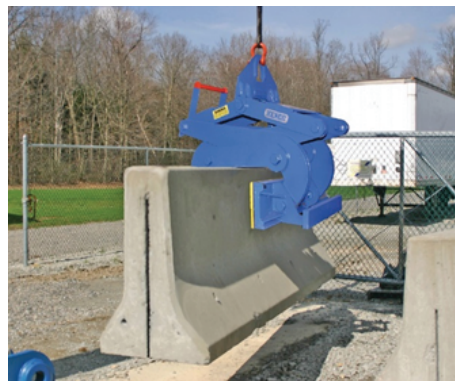
The barrier lift moving a concrete barrier
